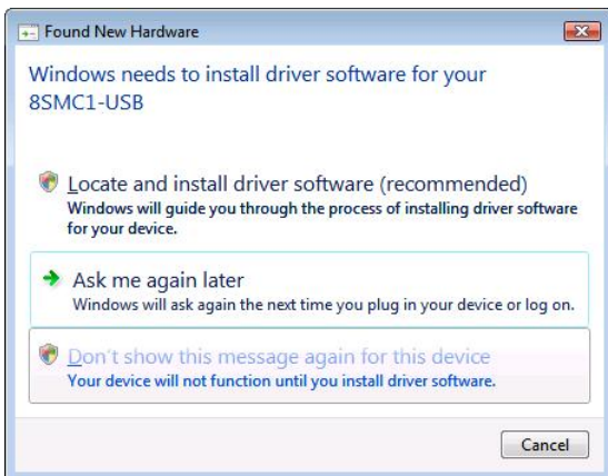
Figure 72. Skip automatic driver installation choosing "Don't show this message again for this device" option.
