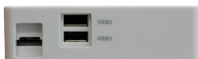
View from the right. Left to right: micro-SD card connector , two USB type A female connectors .
