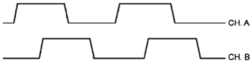
The signals at CH A and CH B outputs of quadrature encoder.
