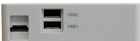
View from the right. Left to right: micro-SD card connector , two USB type A female connectors .
