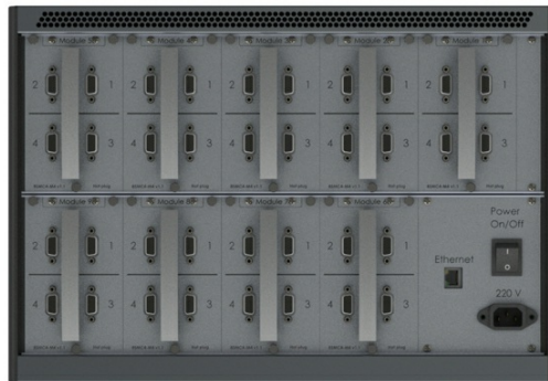
Back view of multi-axis system. View from 220V power connector and control modules side.
